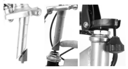
Figure 2a, 2b and 2c. Inserting the handlebar quill into the fork.
